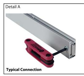
Most horizontal extrusion connections have a patented expandable lock. This lock inserts into the groove of an opposing extrusion. Tightening the lock with the Hex Key Tool expands the lock and creates a strong positive connection.
